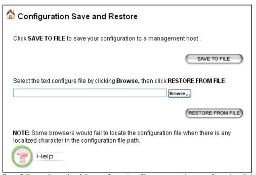
Step 2 Enter the path of the configuration file to save-to/restore-from (or click the **Browse** button to locate the configuration file). Then click the **SAVE TO FILE** button to save the current configuration into the specified file, or click the **RESTORE FROM FILE** button to restore the system configuration from the specified file.
