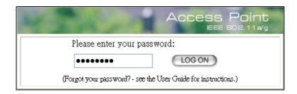
If you are logging on for the first time, you should use the factory default setting "password". The password is always displayed as a string of dots. Click the LOG ON button to start the configuration session.
