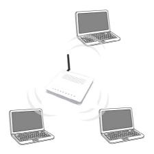
The 802.11A/G ACCESS POINT further provides bridging functions between the wireless network and the wired LAN network.
