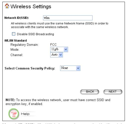
**Network ID (SSID):** The SSID is the network name used to identify a wireless network. The SSID must be the same for all devices in the wireless network (i.e. in the same BSS). Several access points on a network can have the same SSID. The SSID length is up to 32 characters. The default SSID is "wlan".
