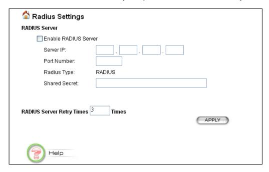
MAC address filtering based authentication requires a MAC address filter table to be created in either the 802.11A/G ACCESS POINT (as described in Chapter 3.2.3 MAC Filtering Settings) and/or the Radius server. During the authentication phase of a wireless station, the MAC address filter table is searched for a match against the wireless client's MAC address to determine whether the station is to be allowed or denied to access the network.
