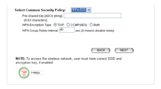
Wi-Fi Protected Access (WPA) with Pre-Shared Key (PSK) provides better security than WEP keys. It does not require a RADIUS server in order to provide association authentication, but you do have to enter a shared key for the authentication purpose. The encryption key is generated automatically and dynamically.
