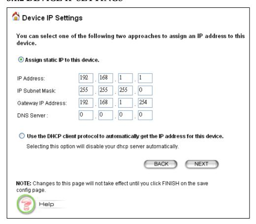
The **Device IP Settings** screen allows you to configure the IP address and subnet of the device. Although you can rely on a DHCP server to assign an IP address to the 802.11A/G ACCESS POINT automatically, it is recommended that you configure a static IP address manually in most applications.
