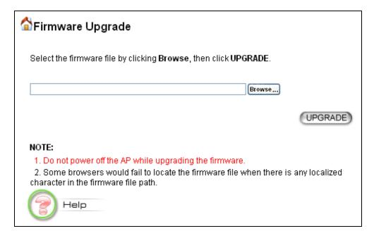
**Step 2** To update the 802.11A/G ACCESS POINT firmware, first download the firmware from the distributor's web site to your local disk, and then from the above screen enter the path and filename of the firmware file (or click **Browse** to locate the firmware file). Next, Click the **Upgrade** button to start.
