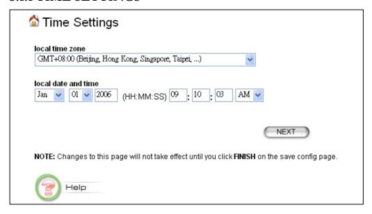
After logging on, the **Time Settings** page appears. The device time is automatically set to the local time of the management PC at the first time a connection is made. To modify the device's time, modify the appropriate fields, then click **NEXT**.
