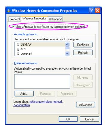
Note: If "Wireless Zero Configuration" is enabled, you can only configure the advance setting or check the link status and statistics from the configuration utility of the card.
