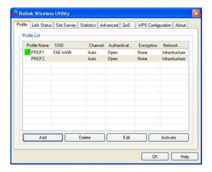
The Ralink Configuration Utility appears as an icon on the system tray of Windows while the adapter is running. You can open the utility by double-click on the icon.
