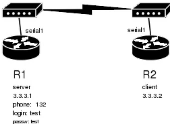
For a typical server setup we need to add one user to the **R1** and configure the PPP server.
